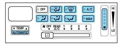
Press AUTOMATIC, any of the override controls or the fan speed control. The EATC will only operate when the engine is running.
